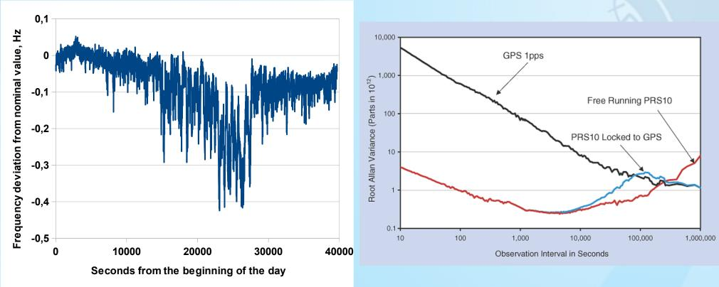
Instantant 10 MHz frequency variation of GNSS receiver within 12 hours, measured by means of the rubidium generator.  $\Delta f l f \approx 1,0E-9.$
