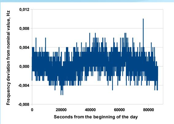
Instantant 10 MHz frequency variation of GNSS receiver within 24 hours, measured by means of the hydrogen generator.  $\Delta f l f \approx 1,0E-10.$
