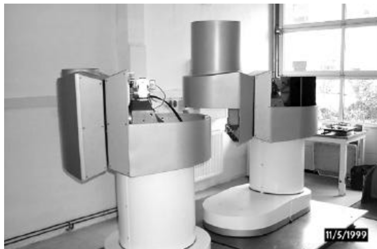
Figure 4.1-6 Close up view of the telescopes in the status of assembling, without optics. Foreground: Transmitter (partially opened) without electronic unit. Background: Receiver, with on the right hand the electronic control unit (black box in the housing).
