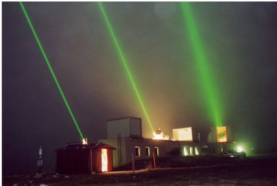
Figure 7.1.2.16-1. Laser Ranging at the Grasse Site.
