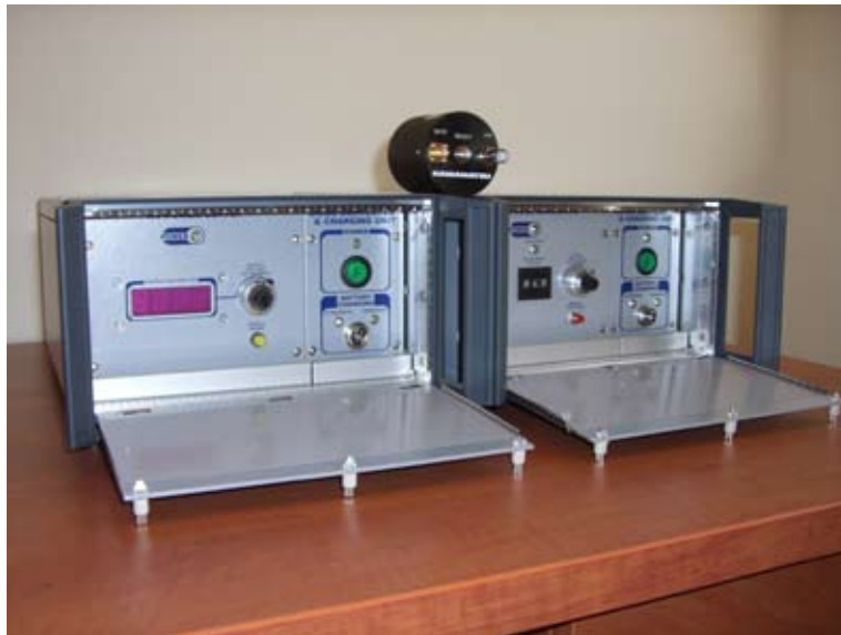
Figure 13-9. MCP-PMT Hamamatsu R5916U-64-3MCP (up), photocathode gating window (right) and power supply (left).
