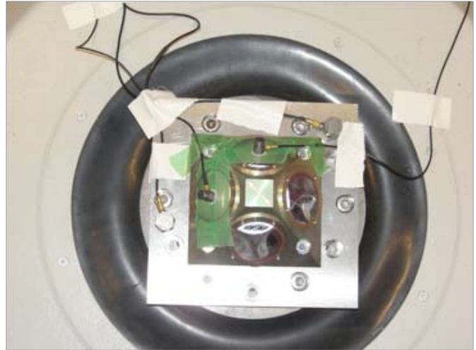
Figure 13-59: LRR array during vibration testing
