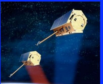
TanDEM-X shall fly in close formation (~300 ... 600 m distance) with TSX to obtain simultaneous X-band radar takes for Digital Elevation Models (DEM)
