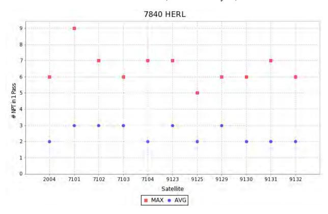
Figure 1-15. Maximum and Average Number of NPT in 1 Pass by HERL for the Second GNSS Campaign; November 24, 2014 - February 28, 2015
