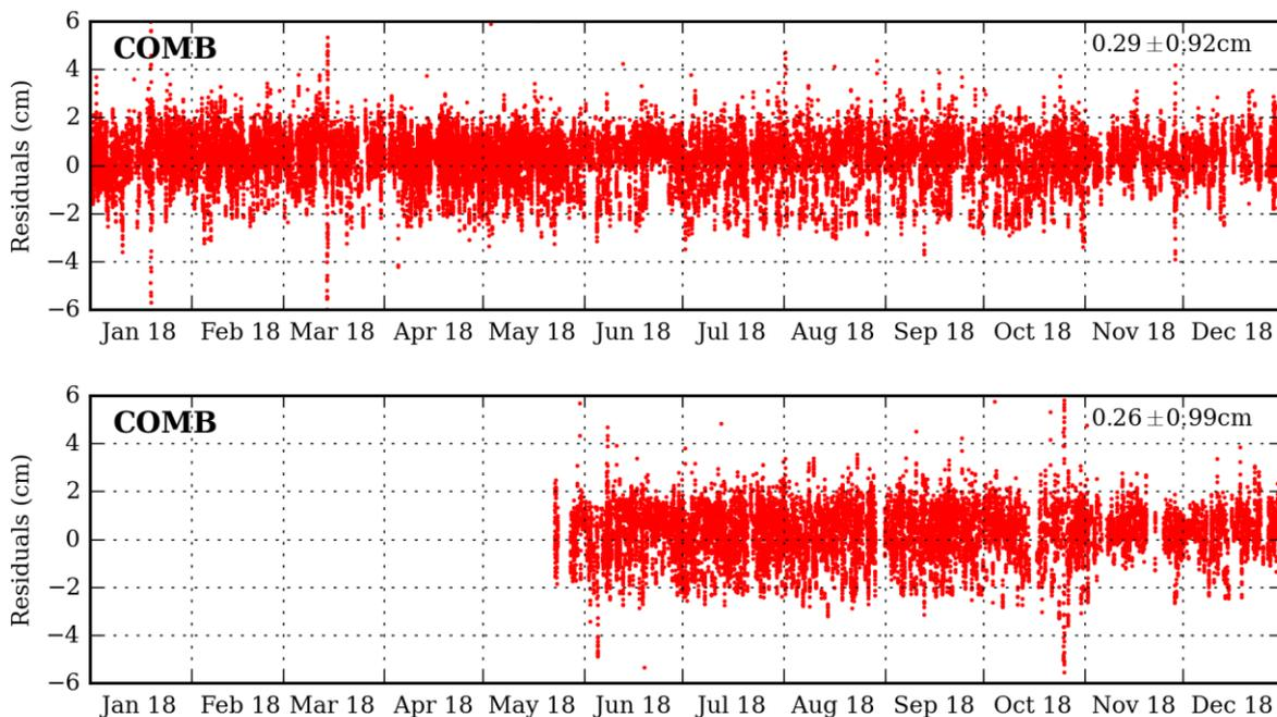
**Figure 3-16: SLR observation residuals of COMB solution for Sentinel-3A (above) and Sentinel-3B (below) during 2018**
