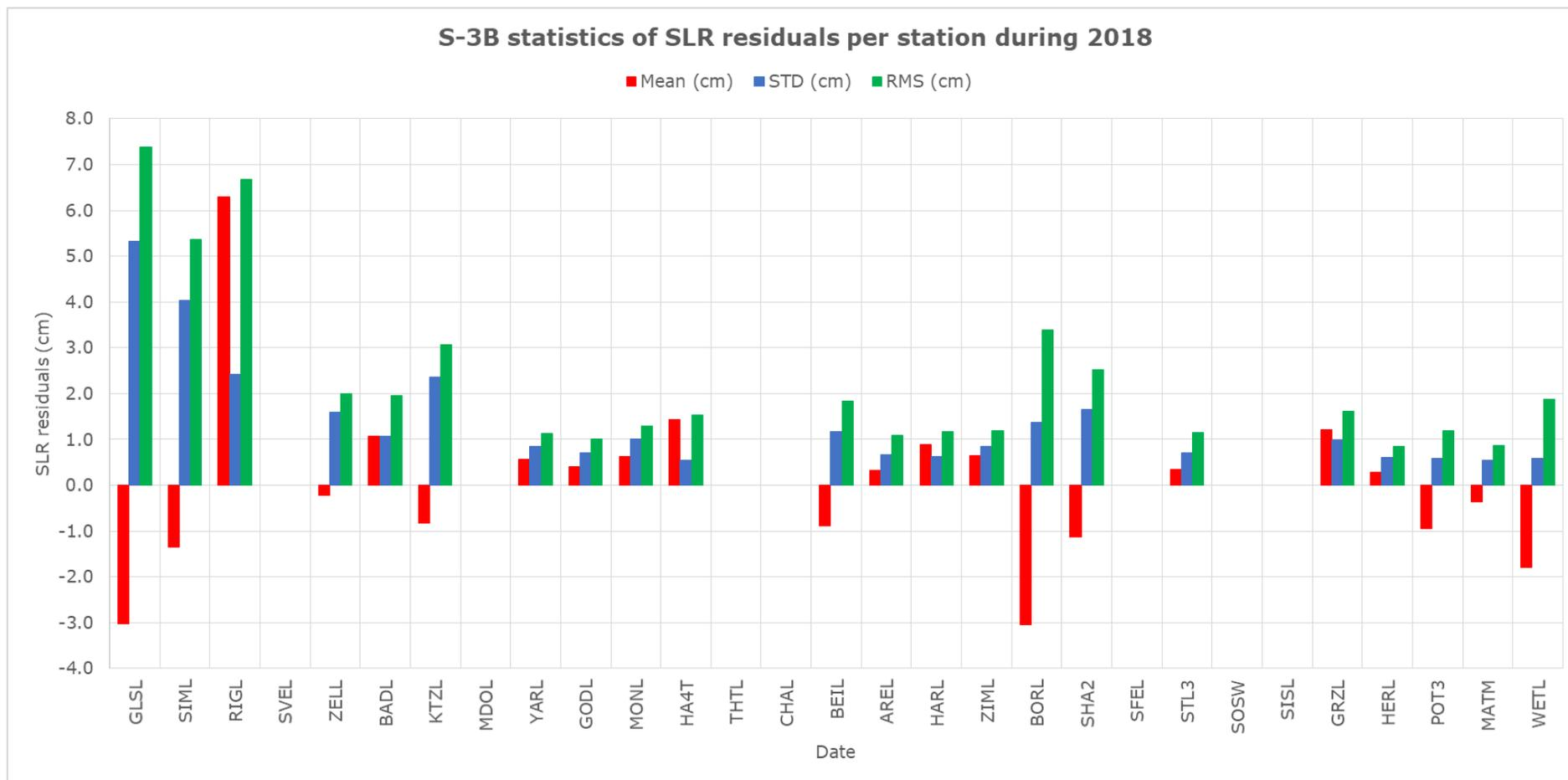
**Figure 3-28: Residuals average, standard deviation and RMS of SLR observations with respect to all stations tracking Sentinel-3B during 2018 (plot)**
