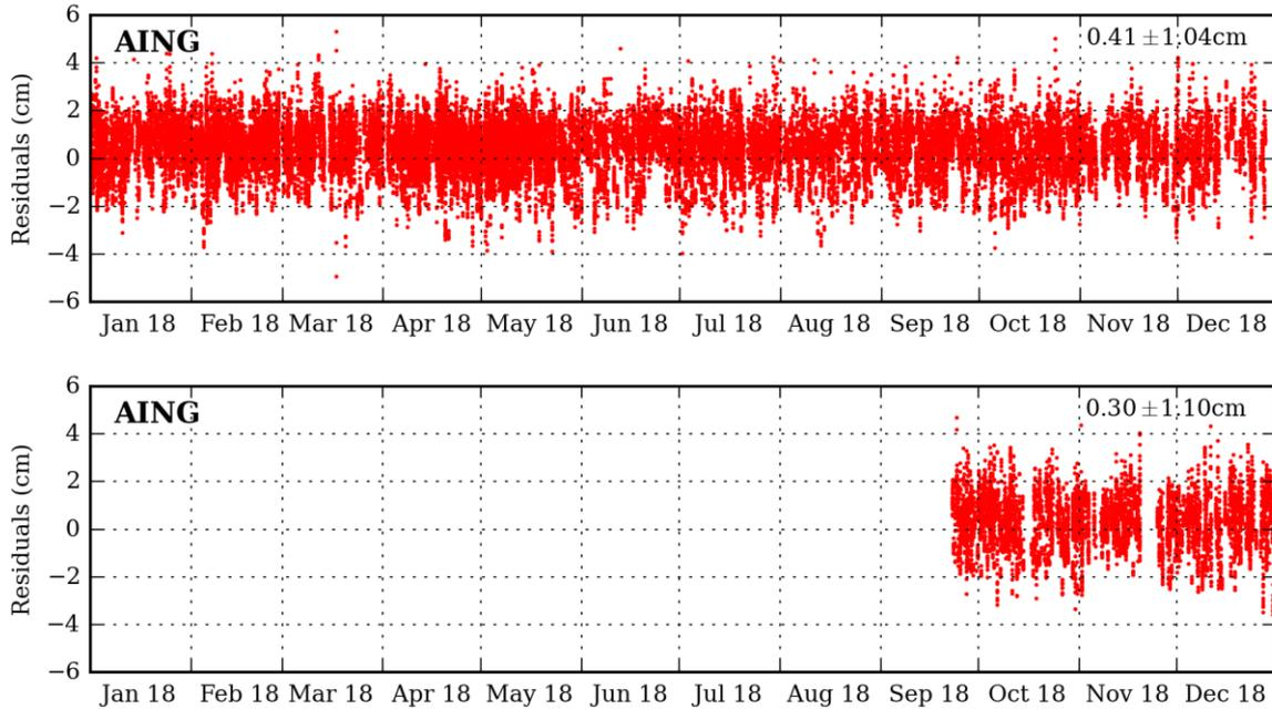
**Figure 3-5: SLR observation residuals of AING solution for Sentinel-3A (above) and Sentinel-3B (below) during 2018**
