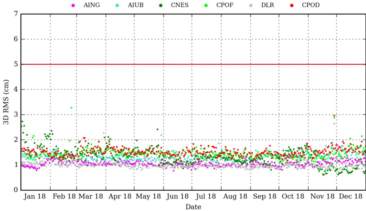
Sentinel-3A Orbital Comparison 3D RMS (cm); COMB vs. external solutions
