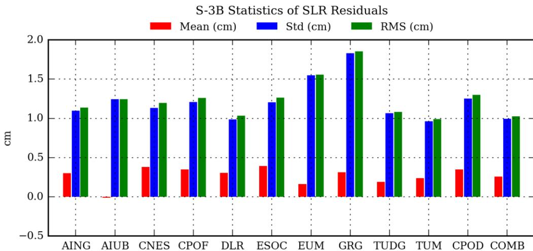
**Figure 3-18: Residuals average, standard deviation and RMS of SLR observations in Sentinel-3B with respect to all orbital solutions during 2018 (plot)**
