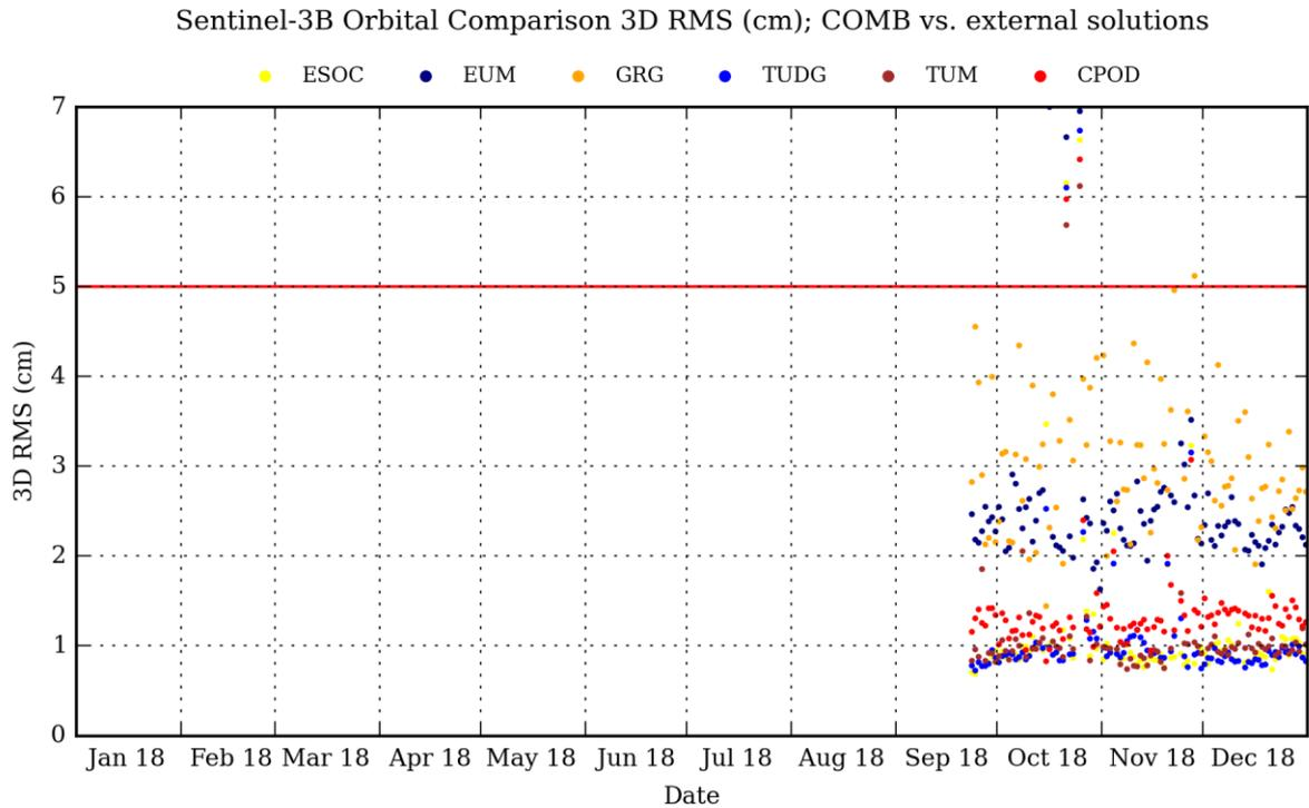
**Figure 3-2: Sentinel-3B orbital comparisons (3D RMS; cm) between COMB orbit and all orbit solutions**
