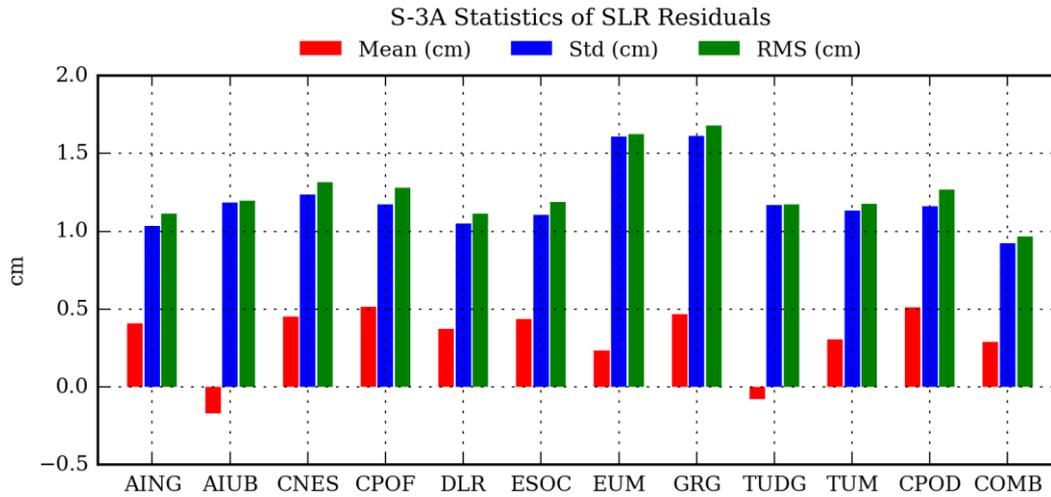
**Figure 3-17: Residuals average, standard deviation and RMS of SLR observations in Sentinel-3A with respect to all orbital solutions during 2018 (plot)**
