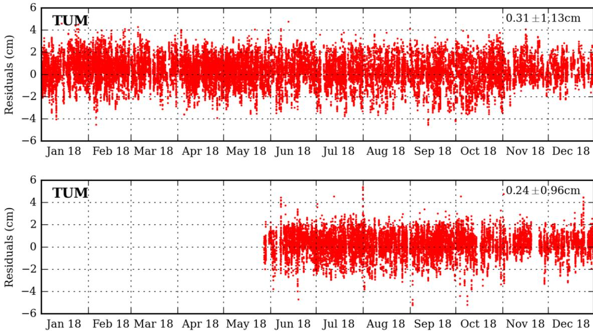
**Figure 3-14: SLR observation residuals of TUM solution for Sentinel-3A (above) and Sentinel-3B (below) during 2018**
