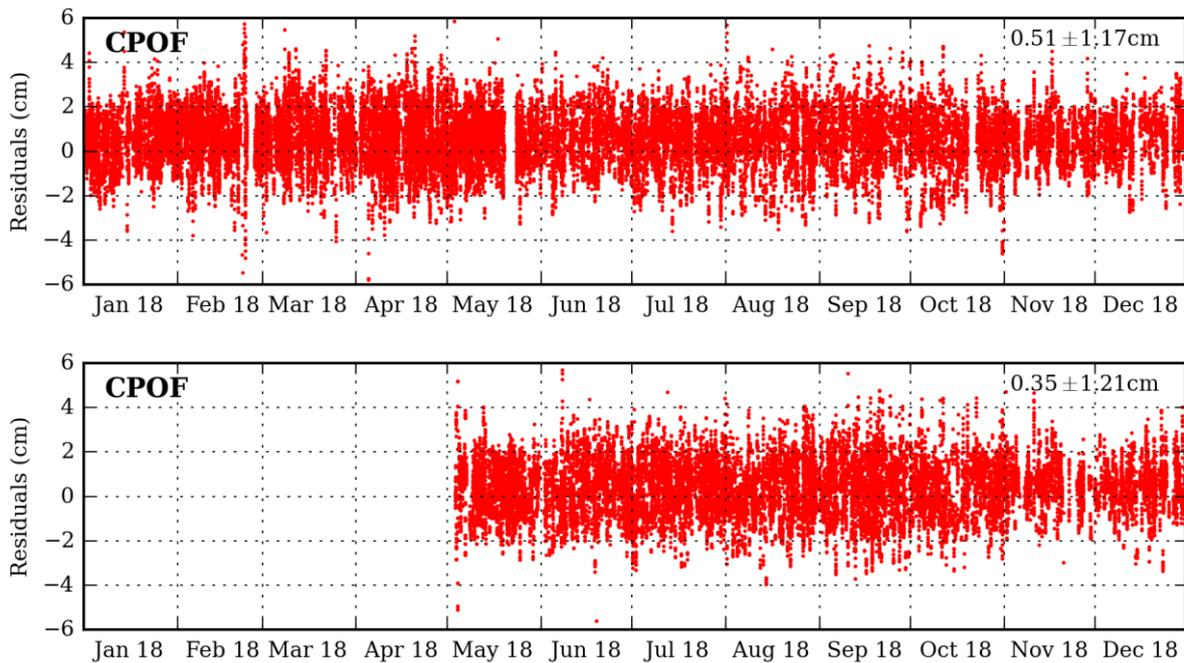
**Figure 3-8: SLR observation residuals of CPOF solution for Sentinel-3A (above) and Sentinel-3B (below) during 2018**
