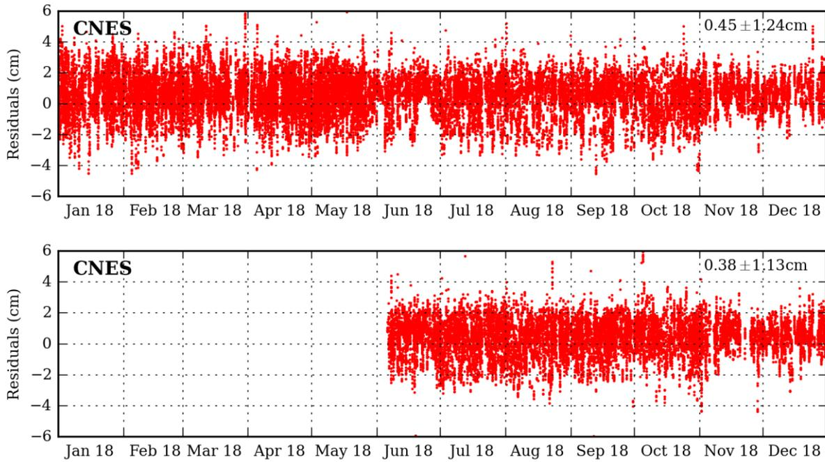
**Figure 3-7: SLR observation residuals of CNES solution for Sentinel-3A (above) and Sentinel-3B (below) during 2018**
