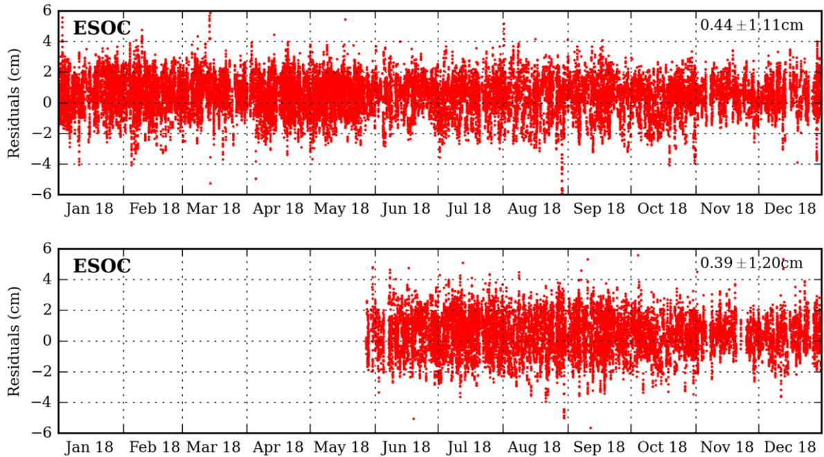
**Figure 3-10: SLR observation residuals of ESOC solution for Sentinel-3A (above) and Sentinel-3B (below) during 2018**
