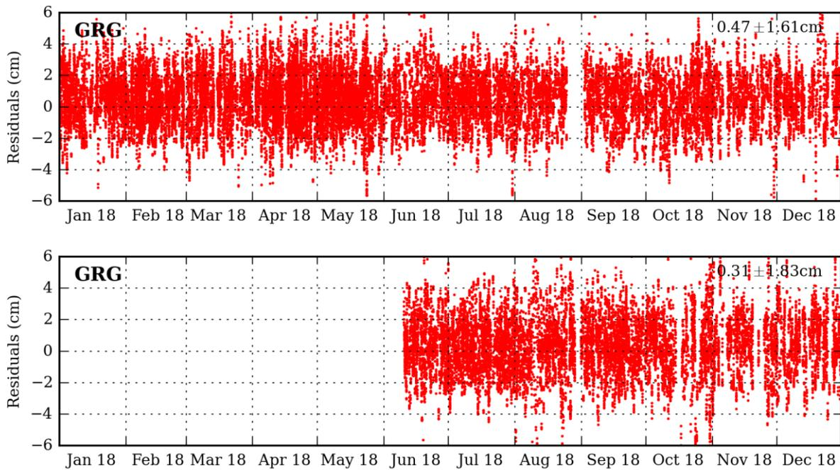
**Figure 3-12: SLR observation residuals of GRG solution for Sentinel-3A (above) and Sentinel-3B (below) during 2018**
