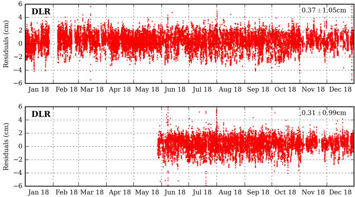
**Figure 3-9: SLR observation residuals of DLR solution for Sentinel-3A (above) and Sentinel-3B (below) during 2018**
