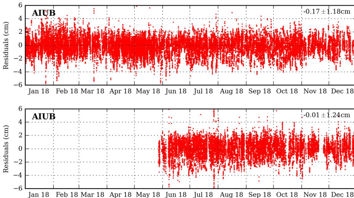
**Figure 3-6: SLR observation residuals of AIUB solution for Sentinel-3A (above) and Sentinel-3B (below) during 2018**
