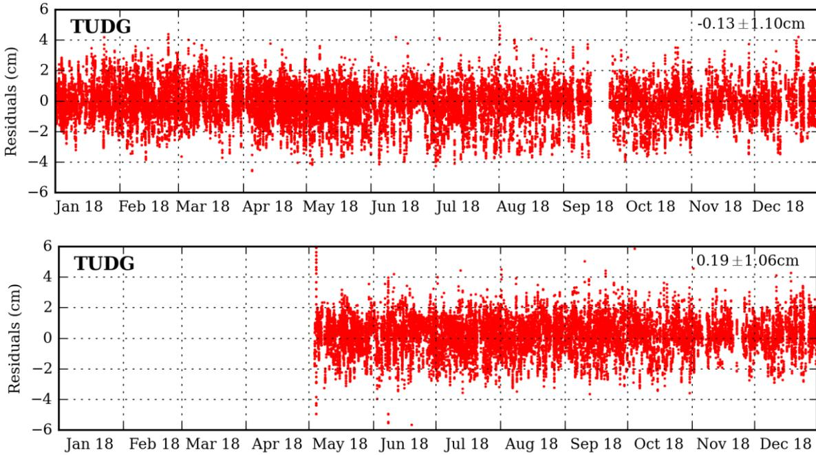
**Figure 3-13: SLR observation residuals of TUDG solution for Sentinel-3A (above) and Sentinel-3B (below) during 2018**
