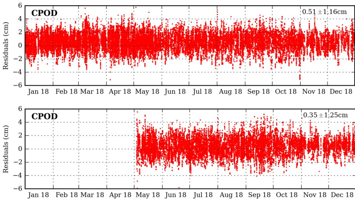
**Figure 3-15: SLR observation residuals of CPOD solution for Sentinel-3A (above) and Sentinel-3B (below) during 2018**
