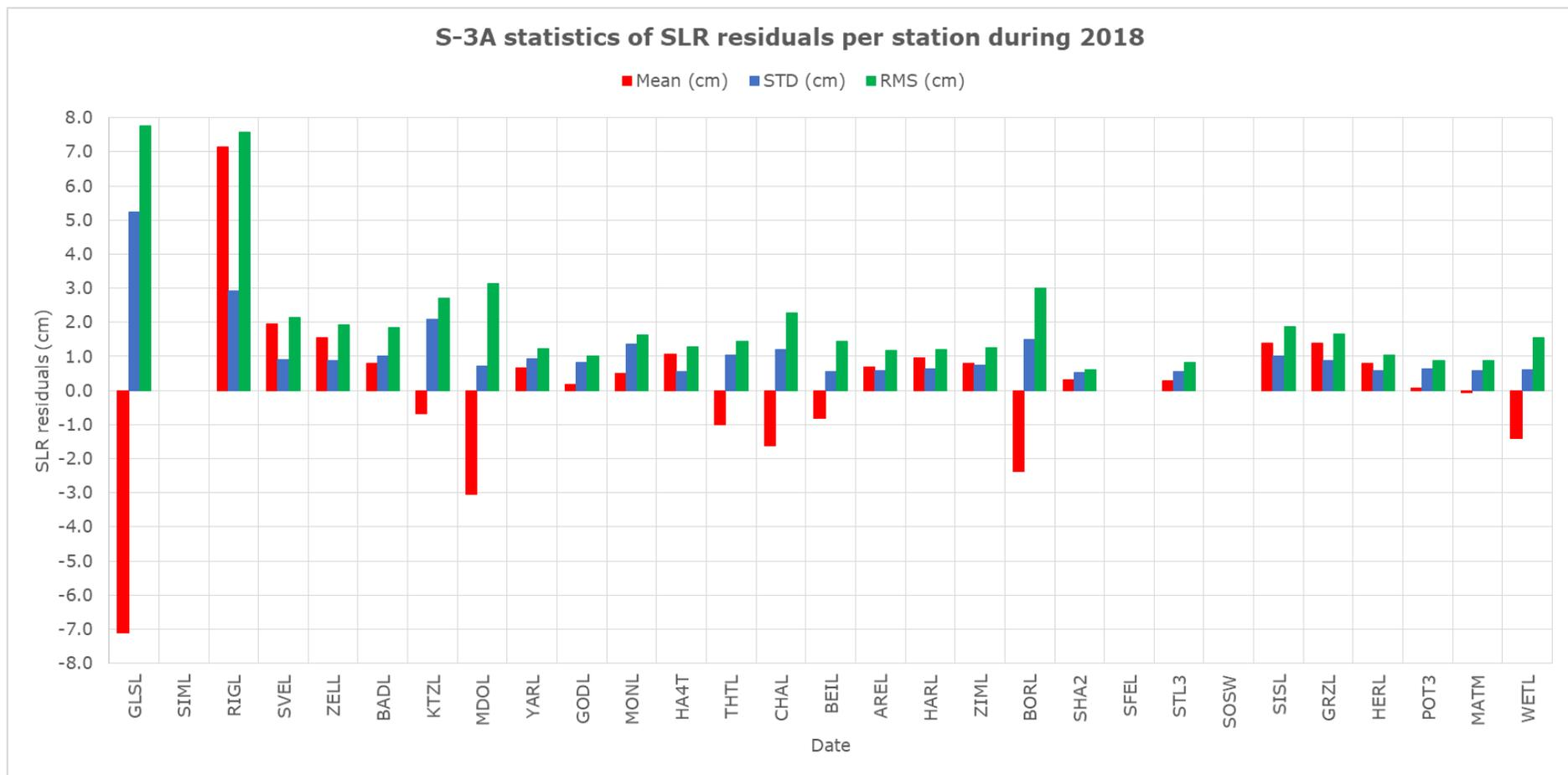
**Figure 3-27: Residuals average, standard deviation and RMS of SLR observations with respect to all stations tracking Sentinel-3A during 2018 (plot)**
