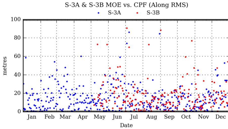
**Figure 4-1: Along RMS for the CPF files vs. MOEORB products during 2018 (Sentinel-3A and Sentinel-3B)**
