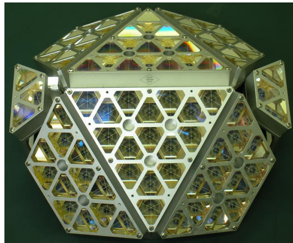
Fig.7 Laser radar retro-reflector array (LRRRA) for TG-2 spacecraft
