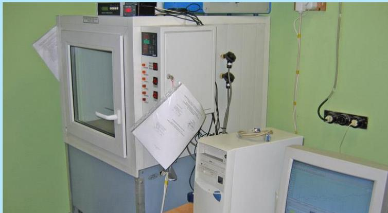
Stationary calibration complex for air temperature sensors
