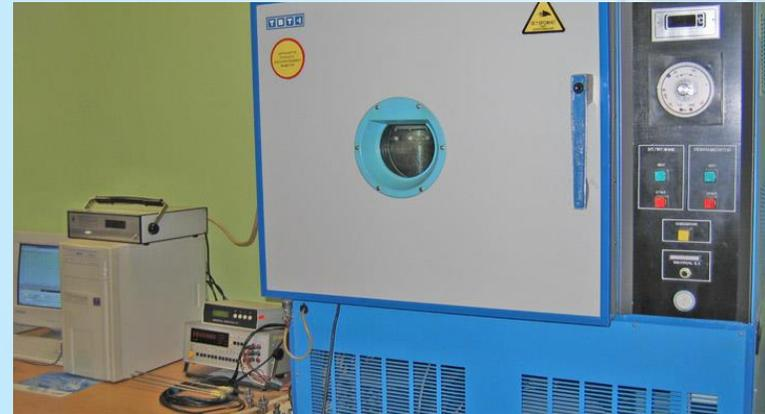
Stationary calibration complex for air humidity sensors
