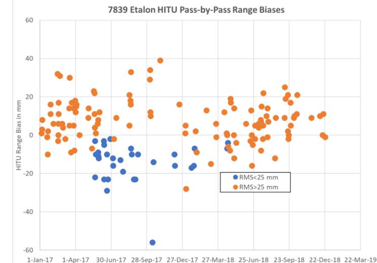
**Left chart:** SSEM 7839 results *Note: The big **highlighted 20 mm** dip in the Etalon bias in mid-2017.*
