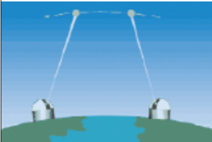
▲ FIGURE 2 SLR provides two-way range measurements from laser stations to satellites carrying laser retroreflector arrays
