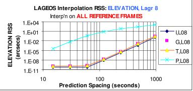
**Figure 1**: Log-log graphs of Range, Azimuth and Elevation Interpolation Errors using an 8<sup>th</sup>-order interpolator in Inertial XYZ (I), Greenwich XYZ (G), Topocentric ENU (T) and local Az/El/R (P) systems.
