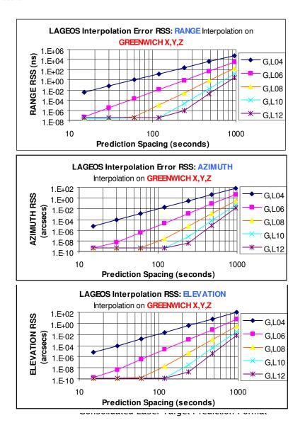
**Figure 2**: Log-log graphs of Range, Azimuth and Elevation Interpolation Errors using interpolators of order 4, 6, 8, 10 and 12 in the Greenwich XYZ (G) system.
