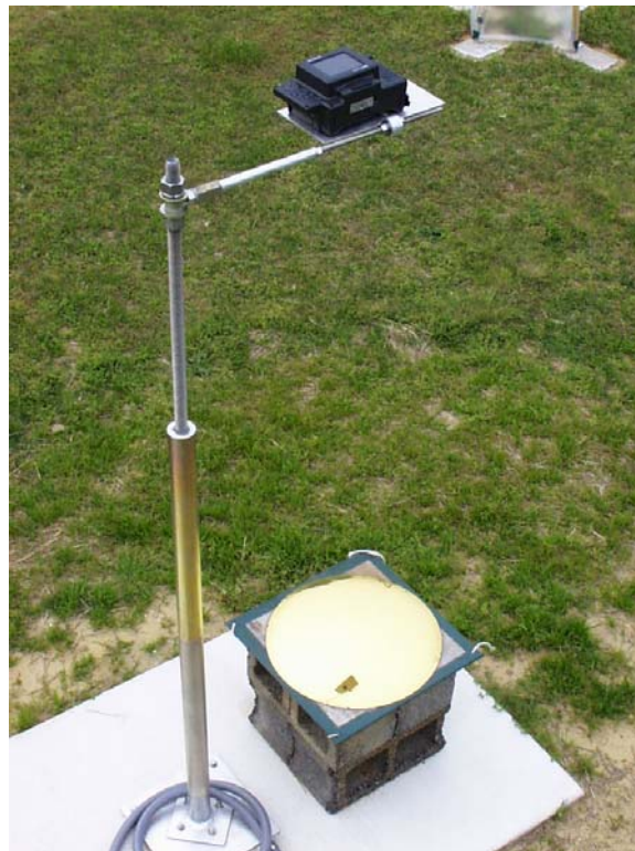
Figure 5: Sky camera and convex mirror
