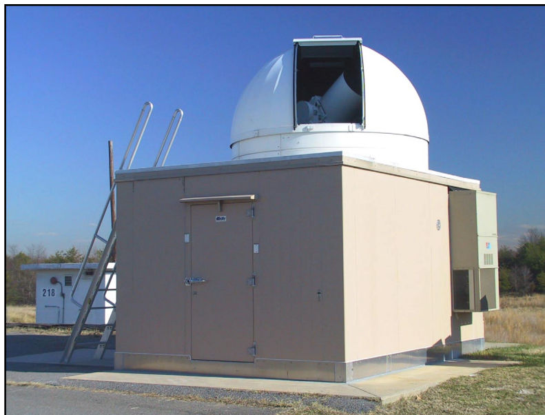
Figure 1: Exterior view of the prototype SLR2000 system with 3 meter tracking dome at the Goddard Space Flight Center. The telescope can be seen in the dome slit.
