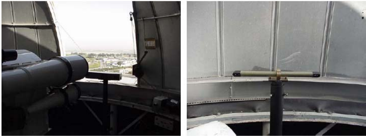
Figure 2: Calibration squares mounted into the telescope dome
