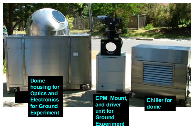
Figure 8: Utility development for Ground outside experiment
