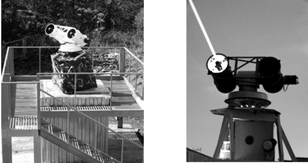
Figure 1: Compact SLR station in operation
