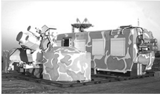
Figure 6: Mobile SLR station installed in Baikonur
