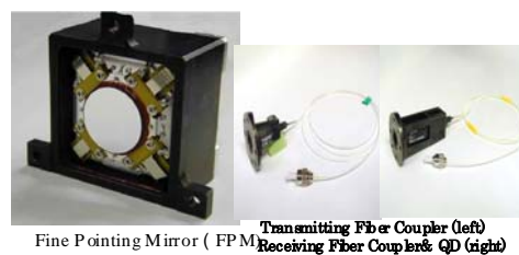
Figure 6: Key components of internal optics
