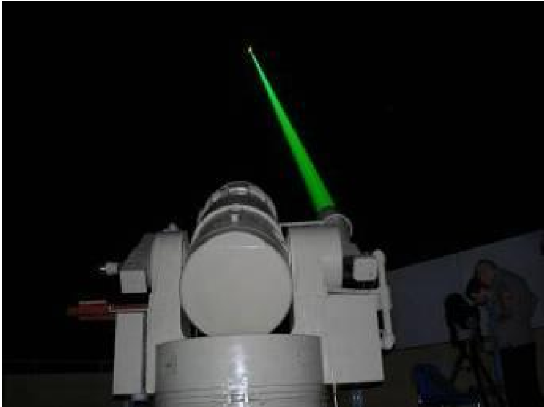
Fig.9. Laser Firing (2J, 20Hz, 40W in 532nm)
