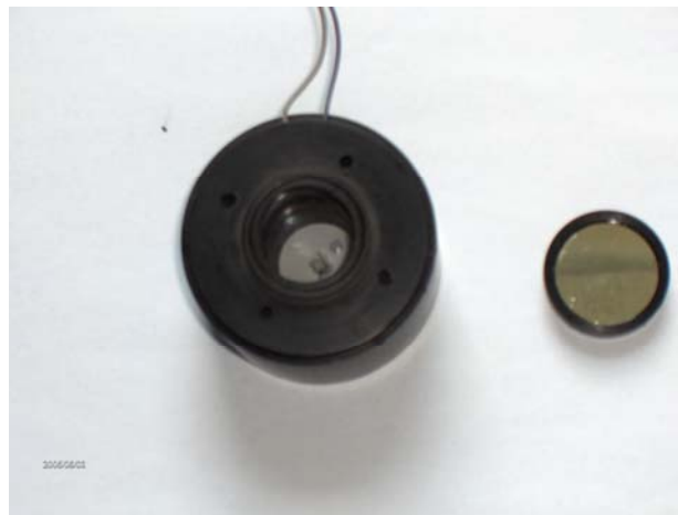
Figure 4. Spectrum filter and constant temperature box
