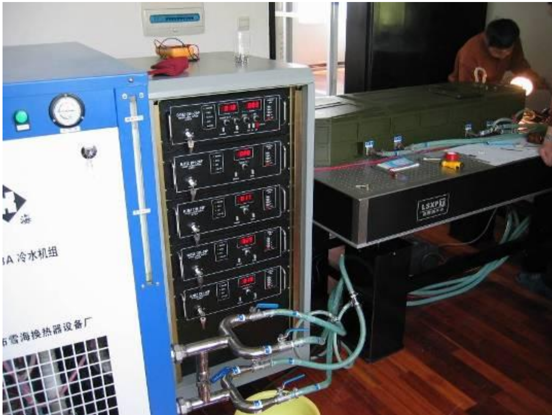
Fig.5. High Power Laser & Power Supply, Chiller
