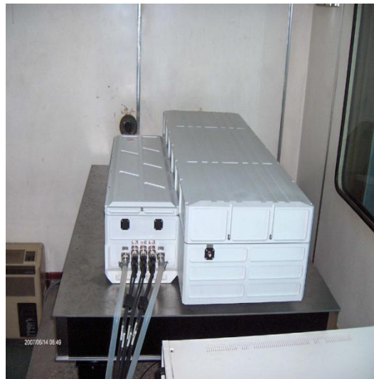
Figure 1. Active-active mode-locked Nd:YAG laser with 100-150mJ (532nm), 250ps,20Hz
