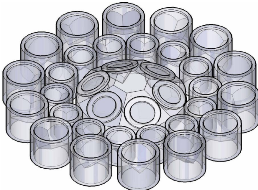
Figure 4. Basic design of ASTRO-G retroreflector array.
