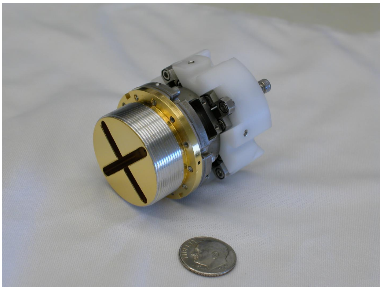
Figure 4. The ANDE Wind and Temperature Spectrometer.
