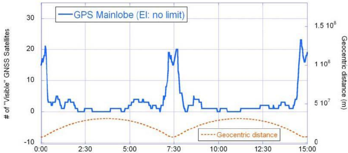
Figure 2. Number of visible GPS satellites
