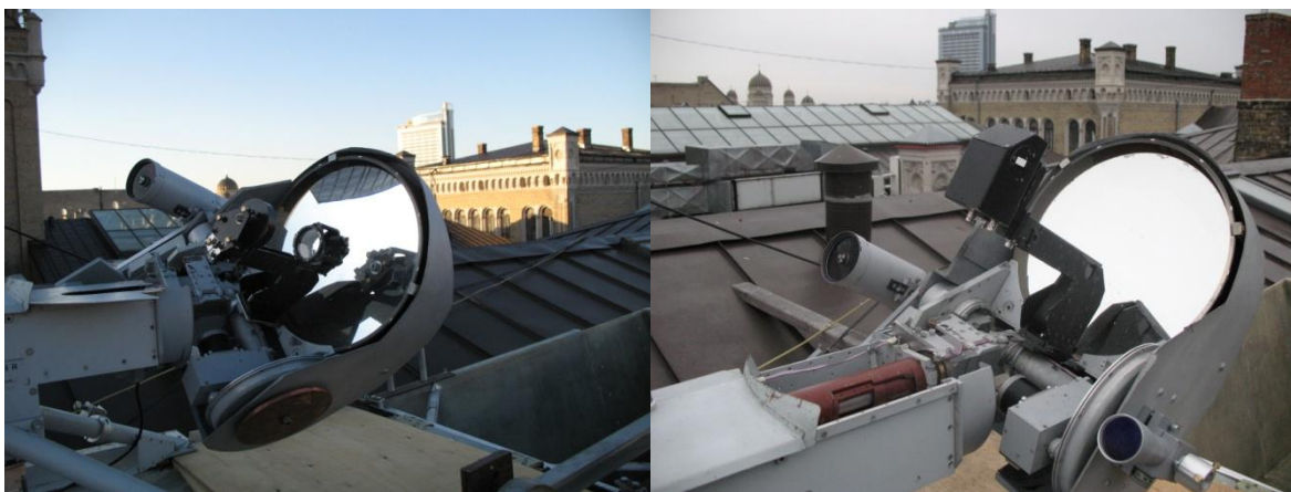
Figure 1. SLR before (left) and after optics modification (right)
