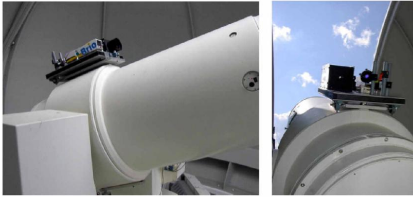
Figure 7. Simulation module mounted on top of the WLRS telescope.
