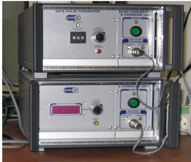
Figure 4. Generator of the gate window (above) and the power supply of MCP-PMT (below).
