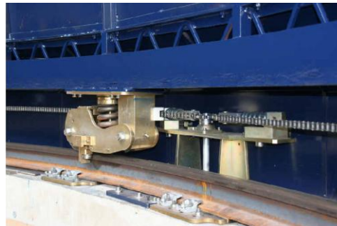
Figure 7. Guiding module of the dome. The rotation is obtained with a 30 meters chain and an asynchronous motor located downstairs
