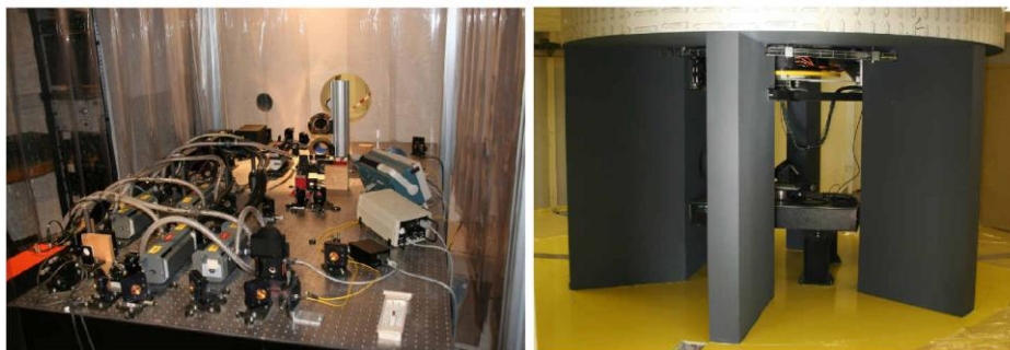
Figure 3. On the left, photography of the laser ranging optical bench. On the right, the pillar of the telescope in the focal laboratory
