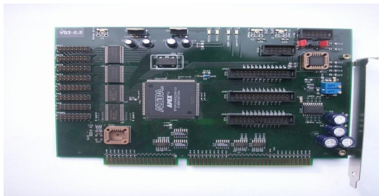
Figure 1. Graz ISA PC Card; FPGA containing Event Timer and Range Gate Generator
