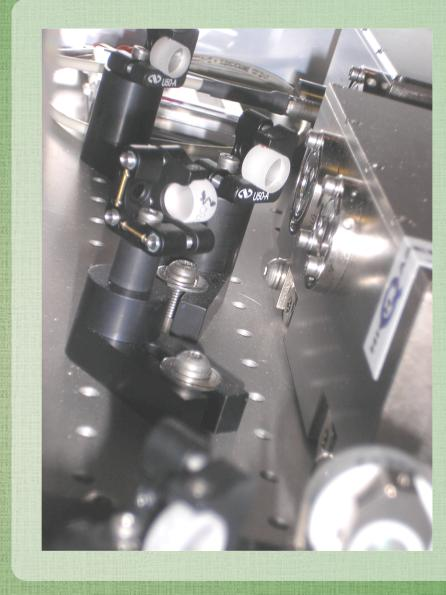
Due to the narrow beamwidth incident at the eyesafe filter, the beam path was increased by about 2m to better disperse the laser energy. This was to avoid critical damage of the ND filters.
