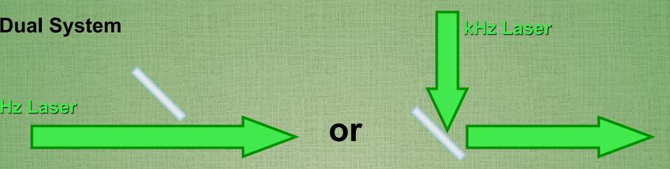
Moveable mirror allows Hz laser through or directs the kHz laser to the coudé path. This is controlled automatically. Alignment between the two lasers must be closely matched.
