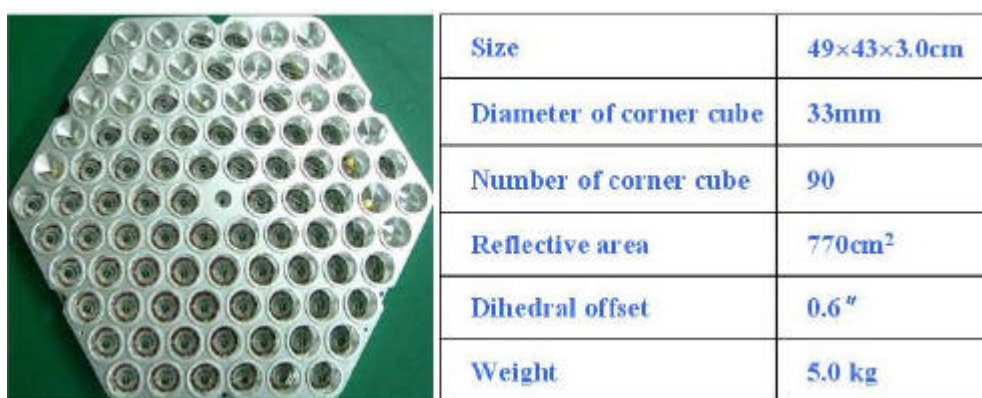
Figure 1 The view of LRA of Compass GEO and IGSO and its main parameters
