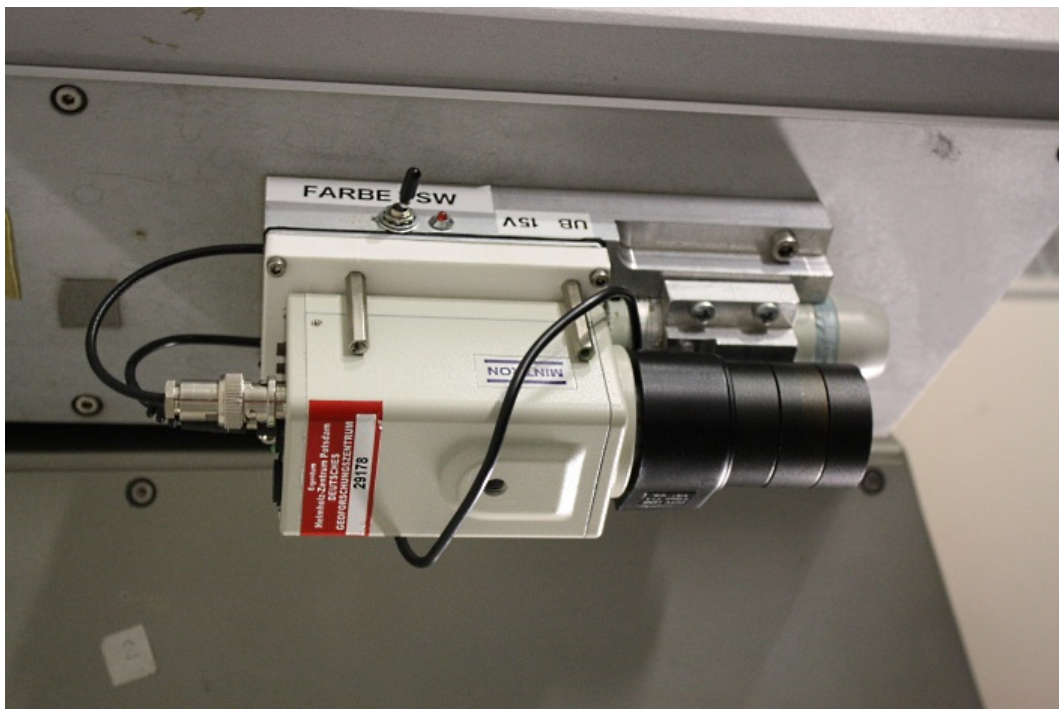
Figure 4. Sky surveillance cameras (stacked B&W and color CCD) on the transmit telescope
