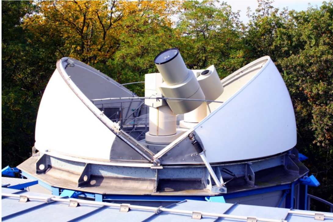
Figure 5. SLR system 7841 Potsdam with separate telescopes for signal transmission and reception
