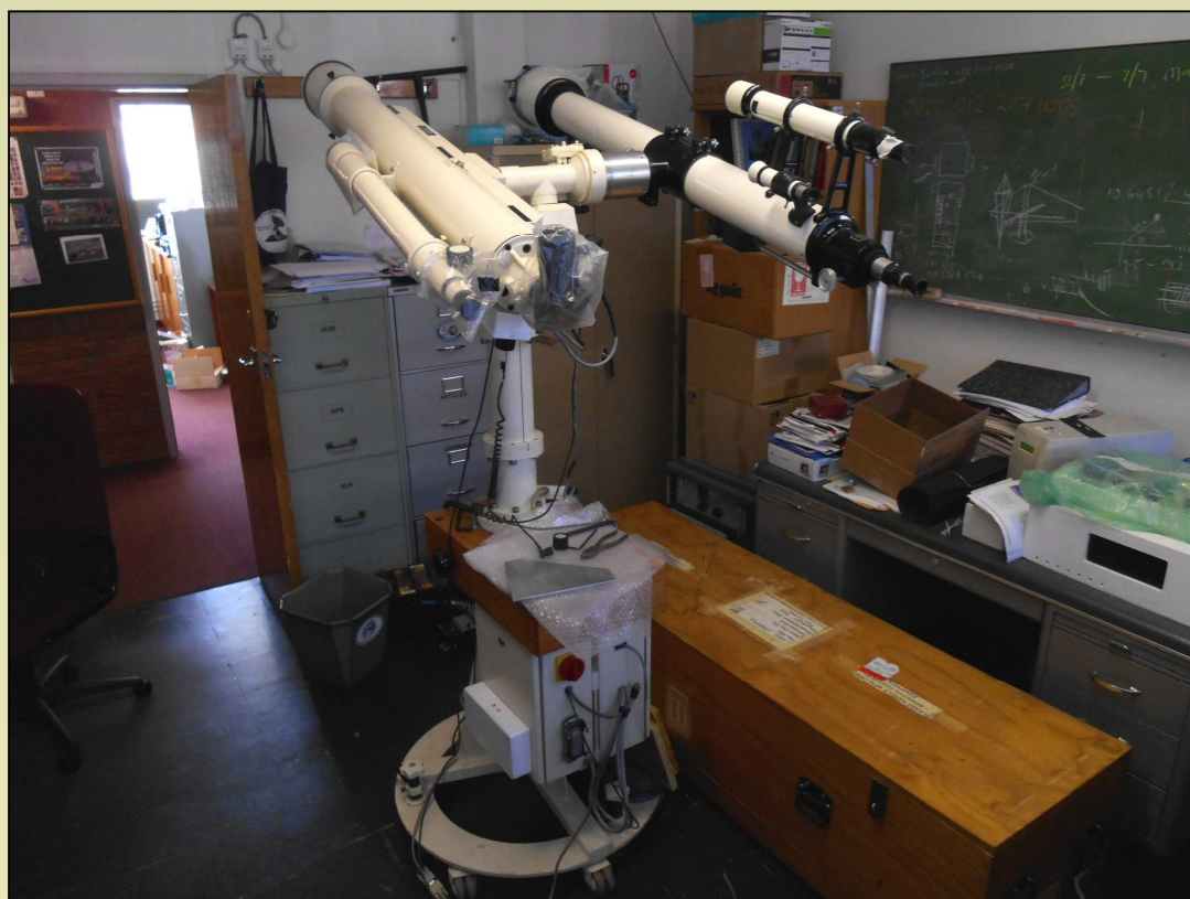
Figure 1. (Left) Small dual refractor used as testbed for the LLR software. Control of relays are done via an ATmega 2560 microcontroller. (Right) Similar control sections will be developed for the LLR telescope.
