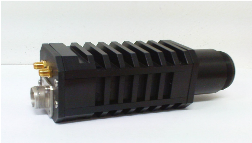
Fig. 1 left - Photograph of SPAD detector package installed in standard housing; right - the PCB of the active quenching and gating circuits.
