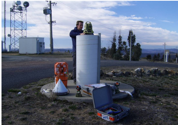
Survey of all calibration targets and fiducial points in local tie network.
