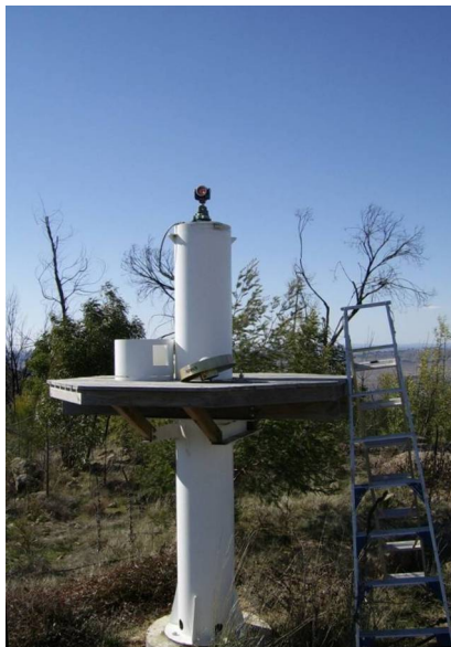
Survey of spigot reference point on calibration pier STN.
