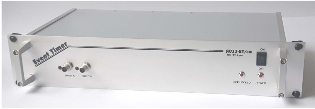
Fig. 1 Event Timer A033-ET in RACK
