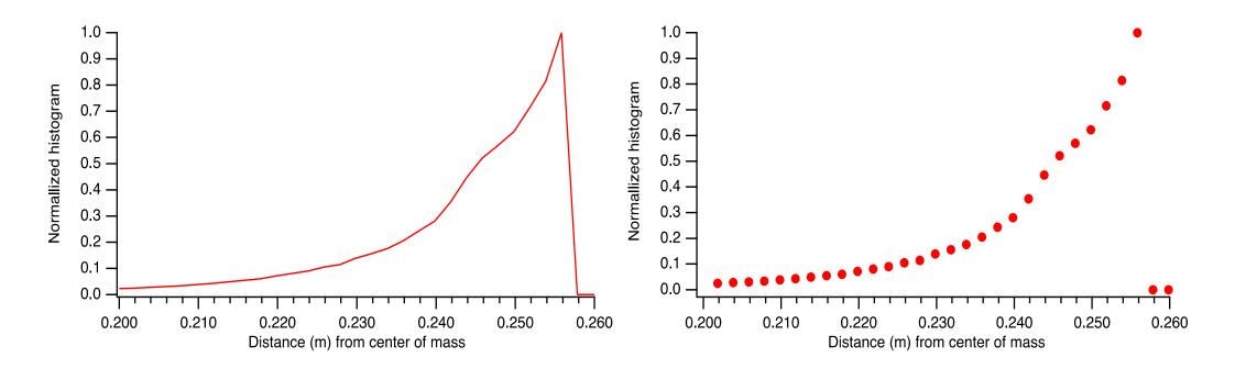
The histogram is obtained by binning data from 2500 incidence angles. The data is the cross section and position along the line of sight for the active cube corners at each incidence angle. Bin size = 2 mm.
