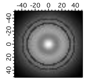
The circles are at the minimum and maximum velocity aberration. The laser receiver is between these two circles at 32 and 40 microradians. The average cross section between the two circles is used as the signal from each cube corner when computing histograms.
